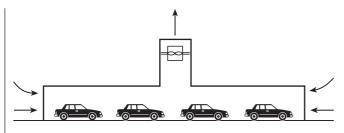
FIGURE I.2.1(e) Longitudinal Ventilation System with Central Fans and Exhaust Shaft.
