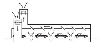
FIGURE I.3.1(a) Full Transverse Ventilation System.
